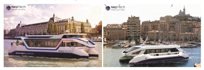
Since May 2020, NepTech has developed its own range of electro-hydrogen-powered vessels from 10 to 30 meters. Its vessels can carry up to 200 passengers or about 20 tons of cargo.
