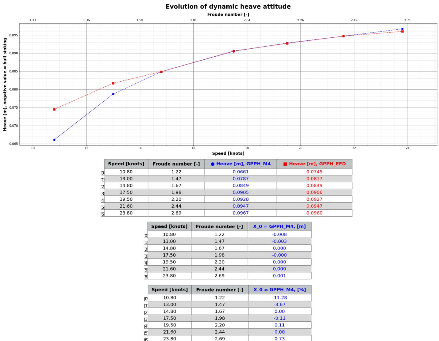
Figure 6: Evolution (up), difference [m] (middle) and difference [%] (bottom) of dynamic heave attitude
